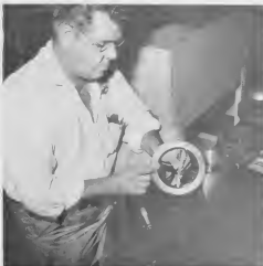
CHIEF INSPECTOR J. M. Bislick gauges an impeller ring from a centrifugal pump. He has 29 years of service. CHIEF INSPECTOR J. M. Bislick ta gauge un impeller ring for di un centrifugal pump. El tin 29 anja di servicio.
